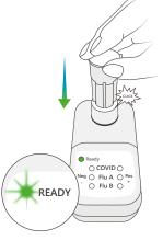
If Ready light is not blinking within 5 seconds, use palm of your hand to press down more firmly to start test.
